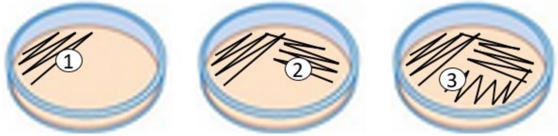
Figure 3.1: Schematic of a Streak Plate Procedure. To streak a plate a sterile inoculum loop is used to gently streak each section starting with the first section and then streaking the next two sections to get three different dilutions of growth on the plate.
